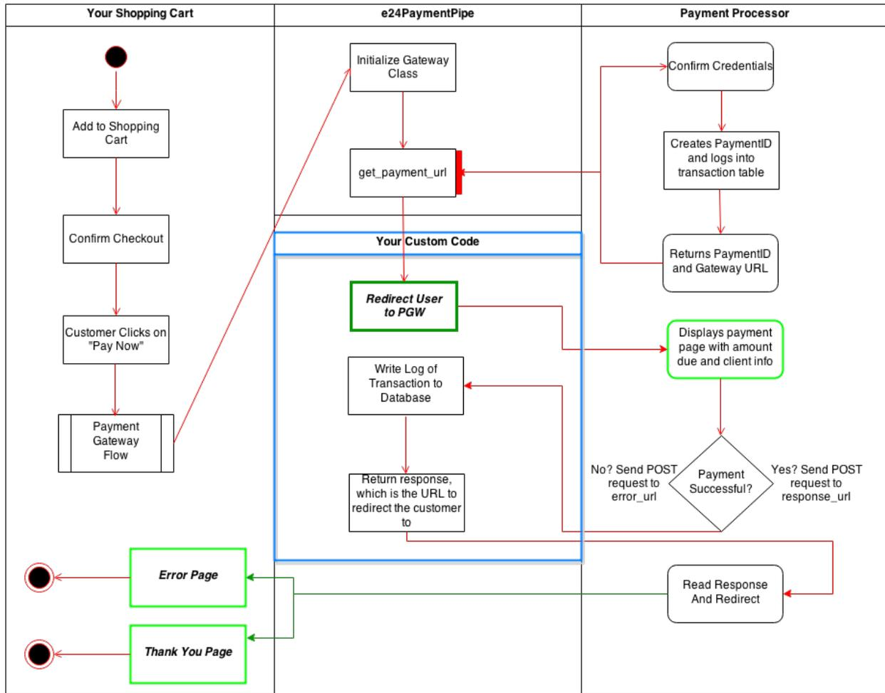
This module provides the functionality contained in the block marked e24PaymentPipe. In a typical use case, you would write the functionality defined in the blue box in order to integrate the payment gateway with an existing system.
